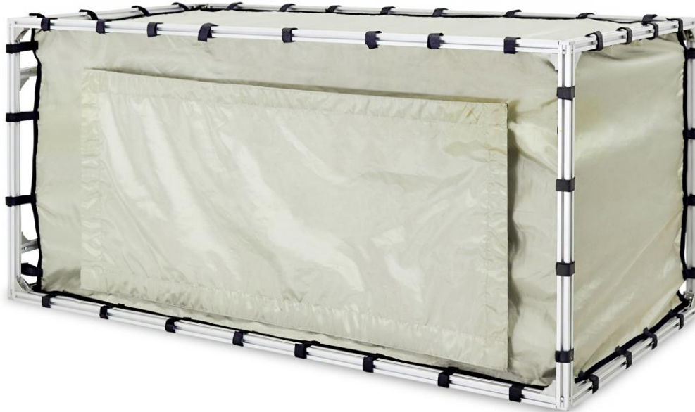
Picture 1: shielded tent with closed opening
